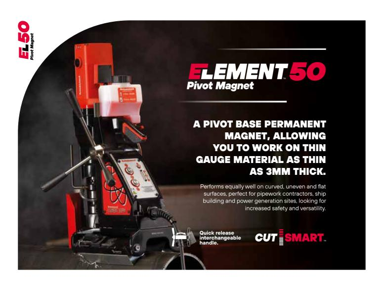
**Cutter Capacity** 50mm 50mm Depth of Cut Twist Drill Capacity 20mm **Drill Chuck Capacity** 13mm MT2 Morse Taper Countersink 30mm M20 Tapping No Load Speed 100-500RPM Motor Specification 1500W 8430N Magnet Adhesion Length 317mm Height 640mm Width 190mm 277 x 190mm Magnet Size **18KG** Weight Motor 110/230V Stroke 150mm
